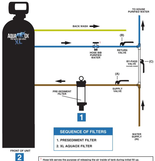
Hose bib serves the purpose of releasing the air inside of tank during initial fill up. Without opening the hose bib to bleed air out, water will only fill up halfway inside the tank, which defeats the purpose of the presoak.
